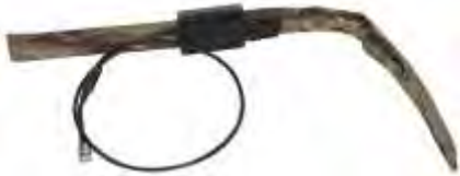
Figure 1. The Harris Dual-Band (UHF and L-band) Antenna is housed in cotton-like webbing that simplifies integration into the warfighter’s kit.
